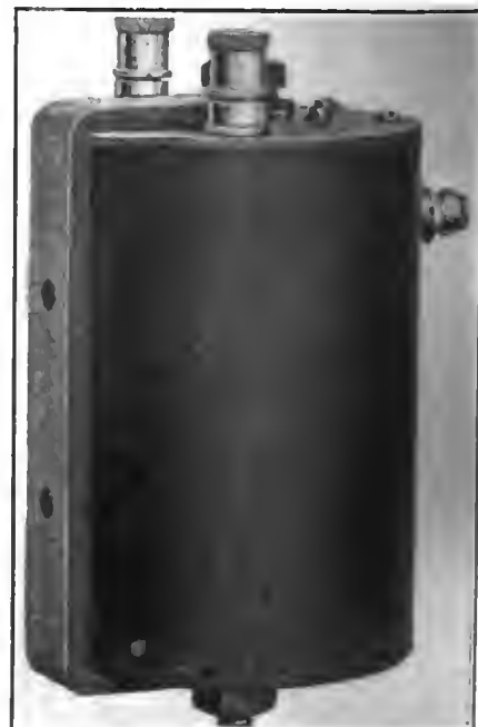
Fig. 5—Distributing coil with the cover removed
